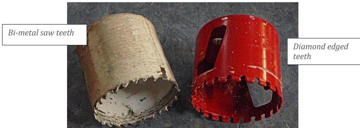
Figure 2 -- Two styles of Hole Saws
