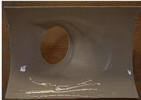
Figure 7 -- PVC Cement freshly applied to GroPocket
