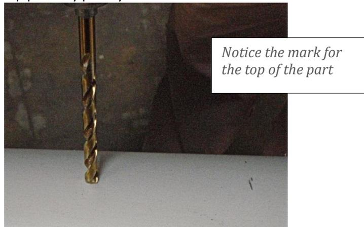
Figure 3 -- Drilling Pilot Hole
